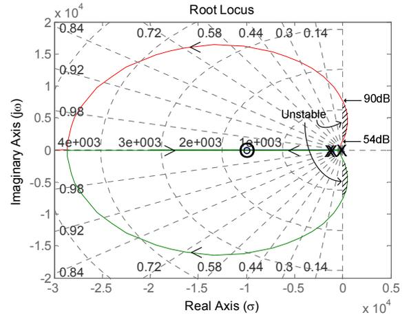
Fig. 2: Root Locus of a 3-pole, 2-zero system.
