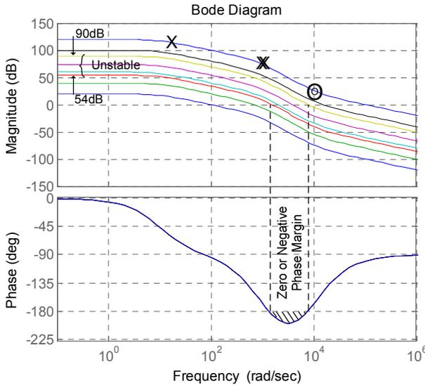
Fig. 1: Bode Plot of a 3-pole, 2-zero system for various values of low-frequency gain  $LG_{FB0}$ .
