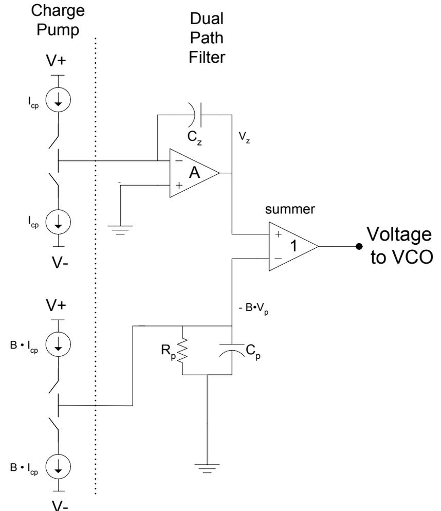
**Method:** Filter cutoff is dependent on switching time, not capacitor size.
