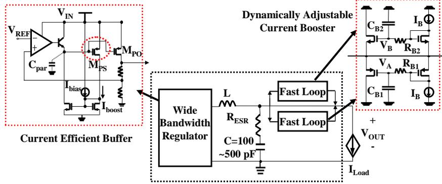
Fully Integrated Regulator For Linear or Switching Regulators
