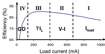
Soft switching + Reduce current ripple to optimize power efficiency !
