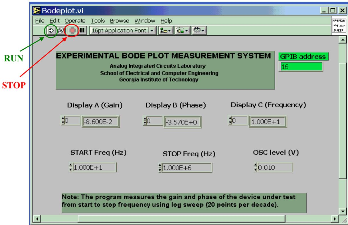
**Step-3:** Enter the values for START Freq, STOP Freq, and the OSC level. The default values are set to be 10 Hz, 10 MHz and 10 mV, respectively. Note that a higher value of OSC output may saturate the amplifiers inside the loop, which yields an incorrect result.
