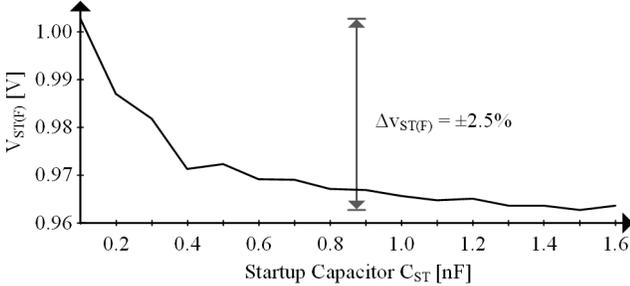
Fig. 8. Measured final startup voltage across  $C_{ST}$ .
