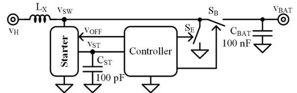
Fig. 2. Proposed self-starting harvester.
