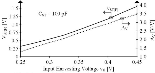
Fig. 7. Measured final startup voltage and gain across  $v_H$ .
