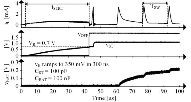
Fig. 11. Measured startup, transition, and steady-state waveforms.
