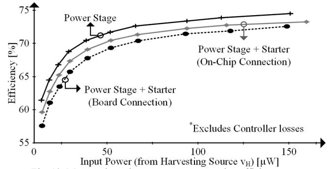
Fig. 12. Measured steady-state power-conversion efficiency.
