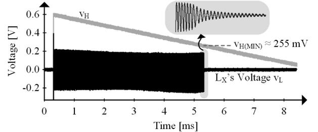
Fig. 6. Measured starter waveforms when  $C_{ST}$  is a pre-charged battery.
