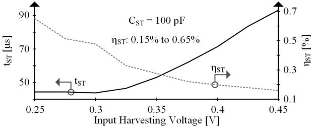
Fig. 9. Measured startup time and conversion efficiency across  $v_H$ .
