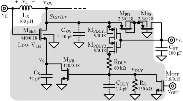
Fig. 3. Prototyped 0.18- $\mu$ m CMOS oscillating starter.
