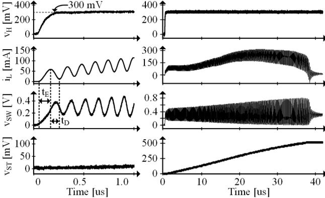
Fig. 4. Measured waveforms of the oscillating starter.
