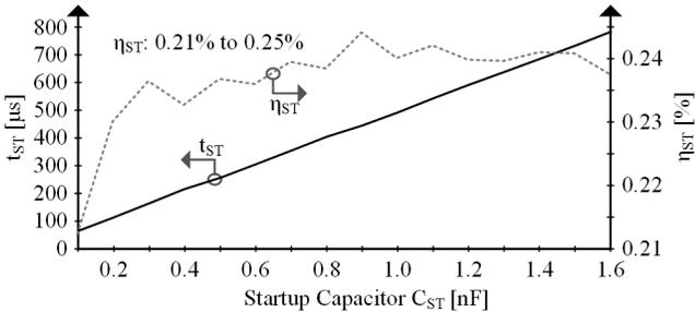
Fig. 10. Measured startup time and conversion efficiency across  $C_{ST}$ .
