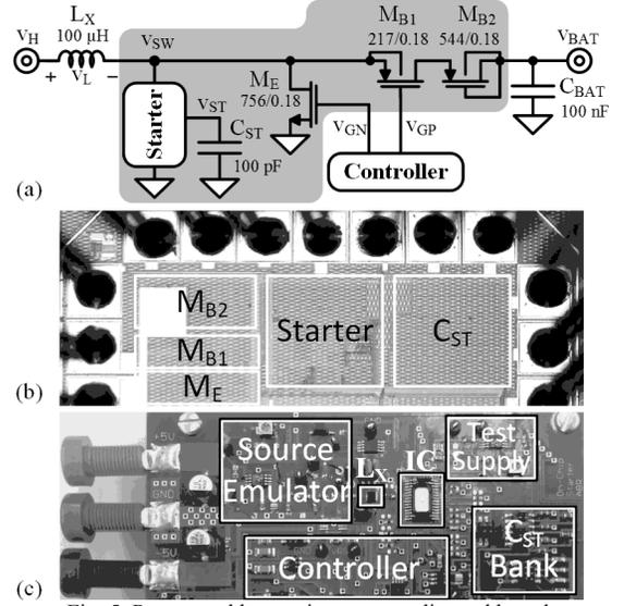
Fig. 5. Prototyped harvesting system, die, and board.
