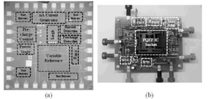
Fig. 7. (a) Die photograph of the  $1.5 \times 1.5 \text{ mm}^2$  energy harvester IC and (b) the printed-circuit board (PCB) used to experimentally test it.
