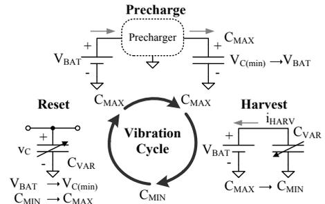
Fig. 1. Energy-harvesting phases: precharge, harvest, and reset [13].
