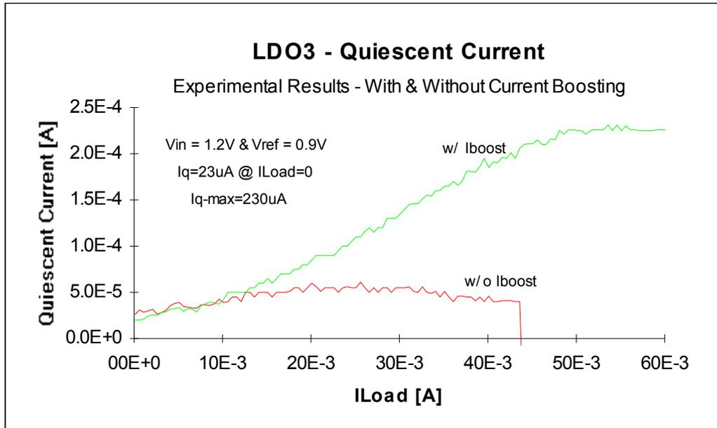
Figure 11. Quiescent current as a function of load-current.
