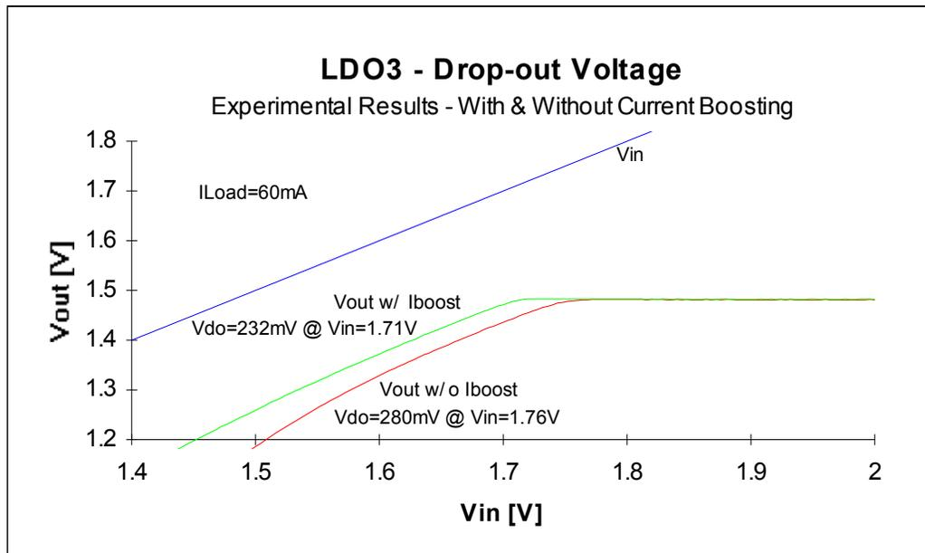
Figure 12. Drop-out voltage performance at 60 mA of load-current.
