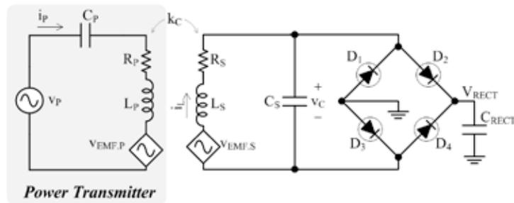
Fig. 2. Resonant power receiver and charger.
