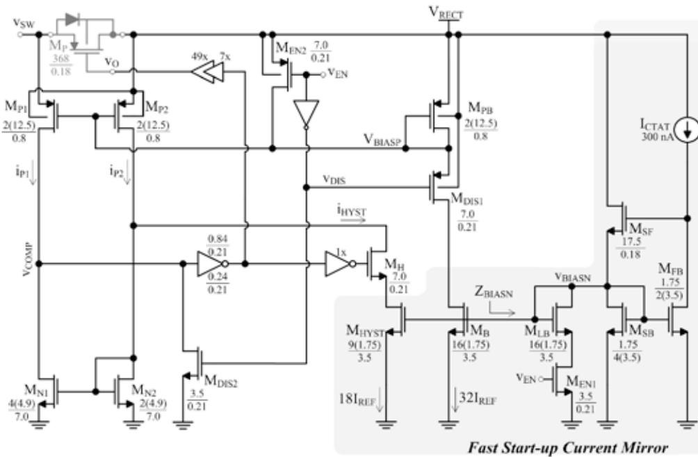
Fig. 7.  $M_P^+$  and  $M_P^-$ 's synchronizing comparator, where n-type bulks are at ground and transistors dimensions are in  $\mu\text{m}$ .
