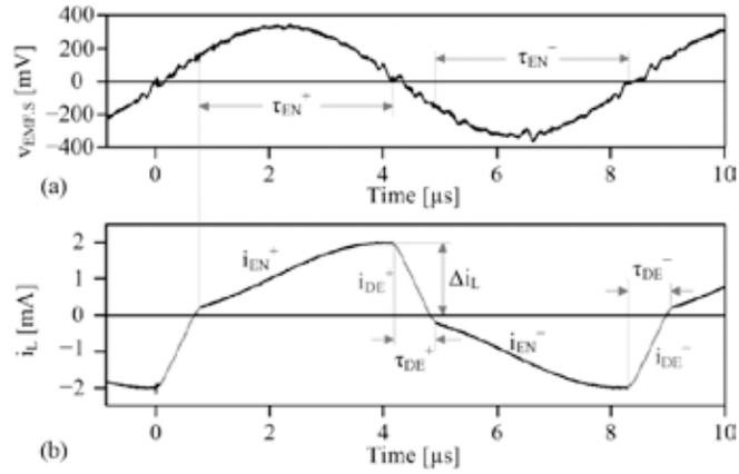
Fig. 4. Measured time-domain waveforms of the receiver coil's (a) EMF voltage and (b) current [35]–[36].
