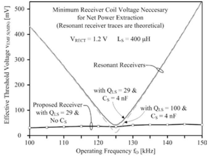
Fig. 12. Measured EMF threshold voltage of the proposed receiver and the theorized counterparts from resonant receivers across frequency.
