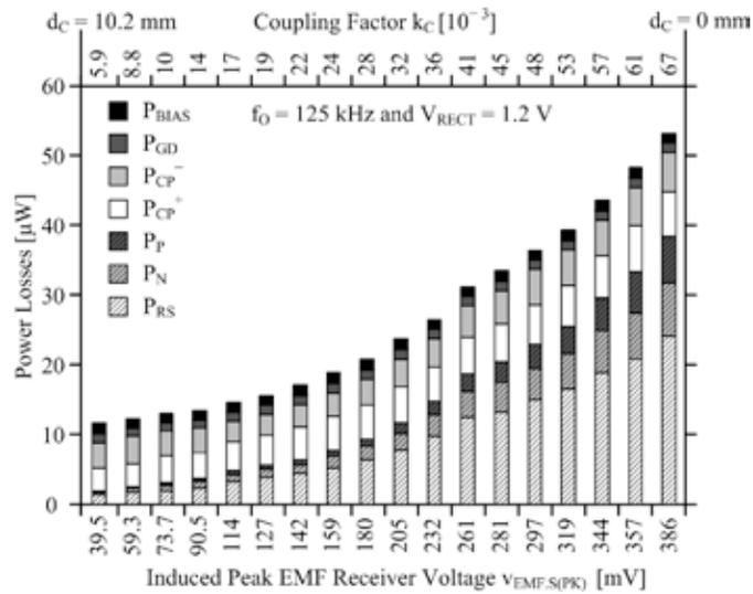
Fig. 13. Measured bias, gate-drive (GD), comparator (CP), p- and n-type switch, and ESR (RS) losses across EMF input power, or equivalently, across  $k_C$ ,  $V_{EMF,S(PK)}$ , and distance  $d_C$ .
