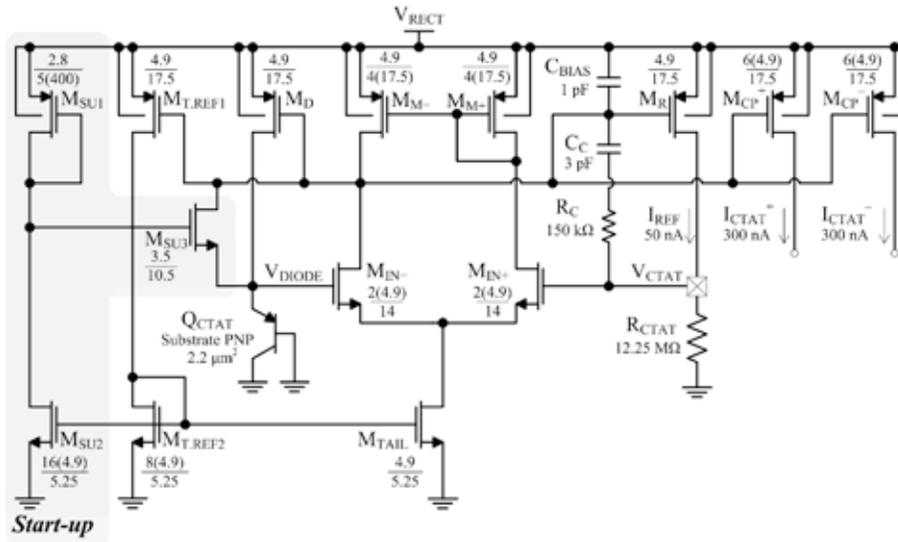
Fig. 8. CTAT current generator, where n-type bulks are at ground and transistors dimensions are in  $\mu m$ .
