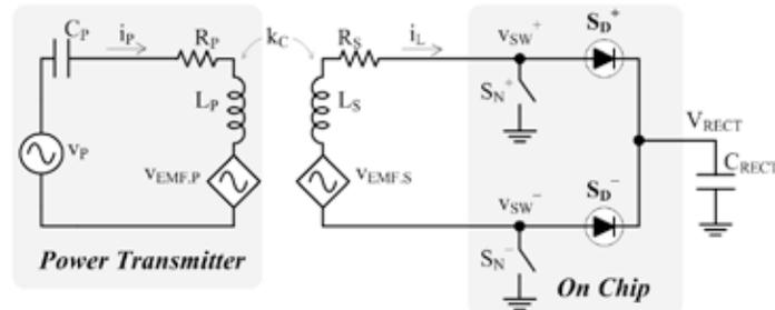
Fig. 3. Proposed switched-inductor power receiver and charger [35]–[36].
