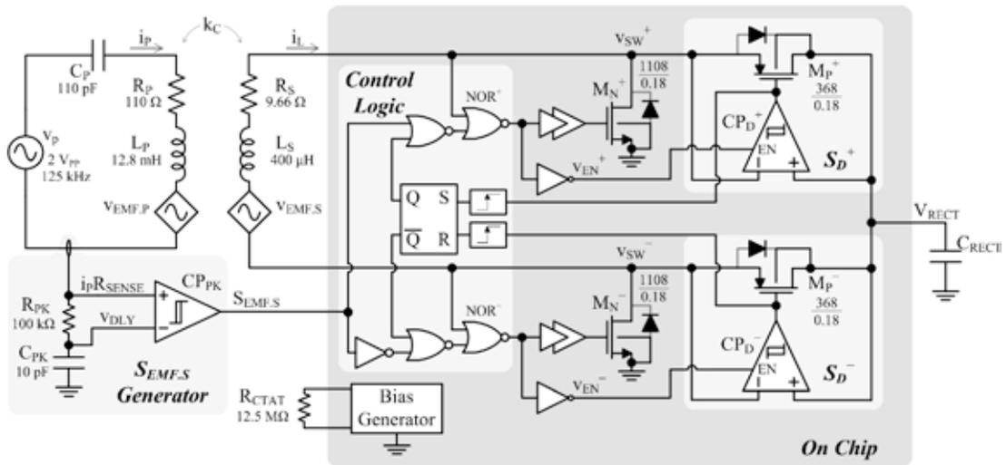
Fig. 5. Prototyped switched-inductor power receiver and charger, where transistor dimensions are in  $\mu\text{m}$ .
