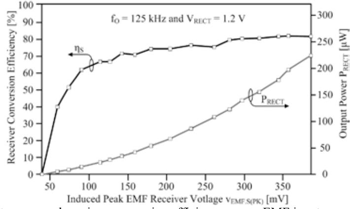
Fig. 14. Measured output power and receiver conversion efficiency across EMF input power, or equivalently, across  $k_C$  and  $v_{EMF.S(PK)}$ .
