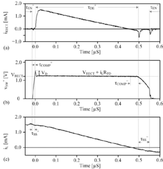
Fig. 6. Measured time-domain waveforms of (a) the rectified current, (b) the positive switching node voltage, and (c) the receiver coil current.
