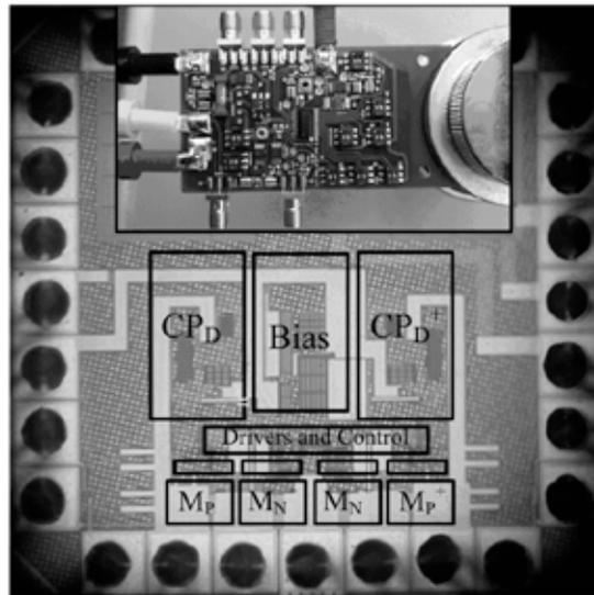
Fig. 9. Prototyped 180-nm CMOS IC and PCB.
