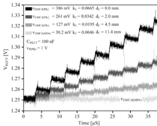
Fig. 11. Measured time-domain charging profiles for a 100-nF SMD ceramic capacitor at 125 kHz.
