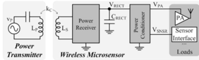
Fig. 1. Wirelessly powering a microsensor system from an inductively coupled source.
