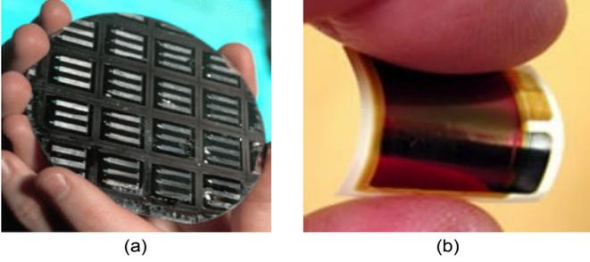
Fig. 2. (a) Micro-scale DMFC and (b) thin-film Li-Ion.
