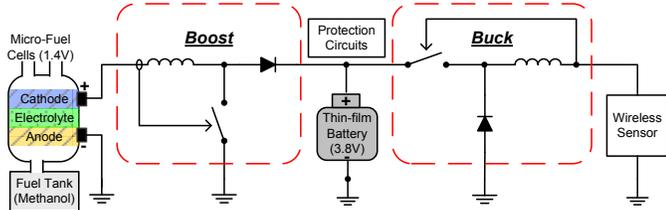
Fig. 5. Hybrid FC-Li-Ion energy- and power-conditioning system.
