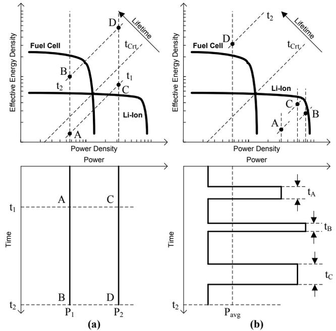
Fig. 4. Energy source mappings for (a) constant and (b) time-dependent loads.
