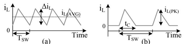
Fig. 2. Inductor-current waveforms in CCM and DCM.
