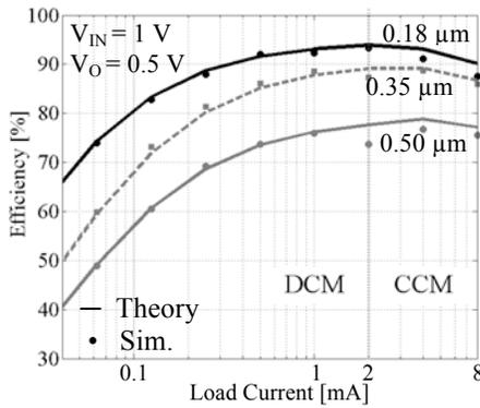
Fig. 6. Efficiency of optimized design across process nodes.
