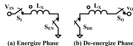
Fig. 1. Alternating (a) energize and (b) de-energize cycles.
