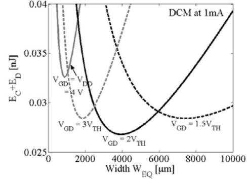
Fig. 7. Losses across width and gate-drive voltages in DCM.
