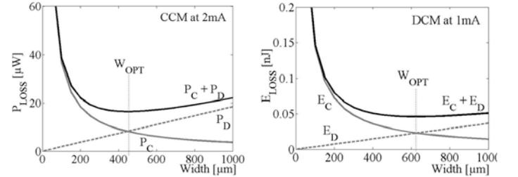
**Fig. 4.** Switch losses across channel widths.
