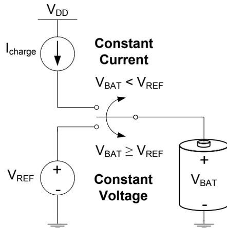
Figure 7. Constant-current/constant-voltage model.
