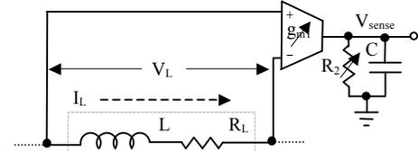
Fig. 1. Block diagram of Current-sensing filter technique.
