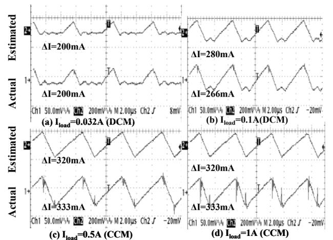
Fig. 9. Estimated and actual ac inductor currents during normal operation and under various loading conditions.
