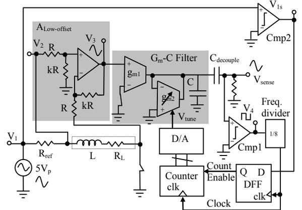
Fig. 5. Tuning circuit.
