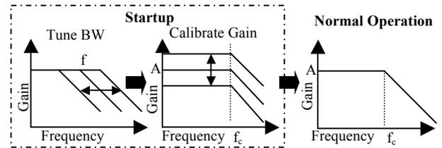
Fig. 2. Proposed start-up sequence: tuning, calibration, and normal operation.
