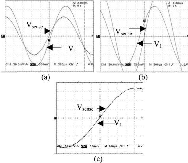
Fig. 6. Output  $V_{sense}$  versus reference  $V_1$  phase response at  $f_{ref}=300\text{Hz}$  with (a) maximum, (b) minimum, and (c) tuned  $g_{m2}$  values.
