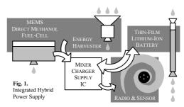
that combine the complementary advantages of evolving Li-Ion, fuel-cell, and harvesting technologies, as shown in Fig. 1, to extend operational life to practical levels. The driving idea is to exploit the power-delivery advantages of Li Ion batteries and extend their life by drawing energy from fuel cells and mixing it with ambient energy harvested from the surrounding environment.
