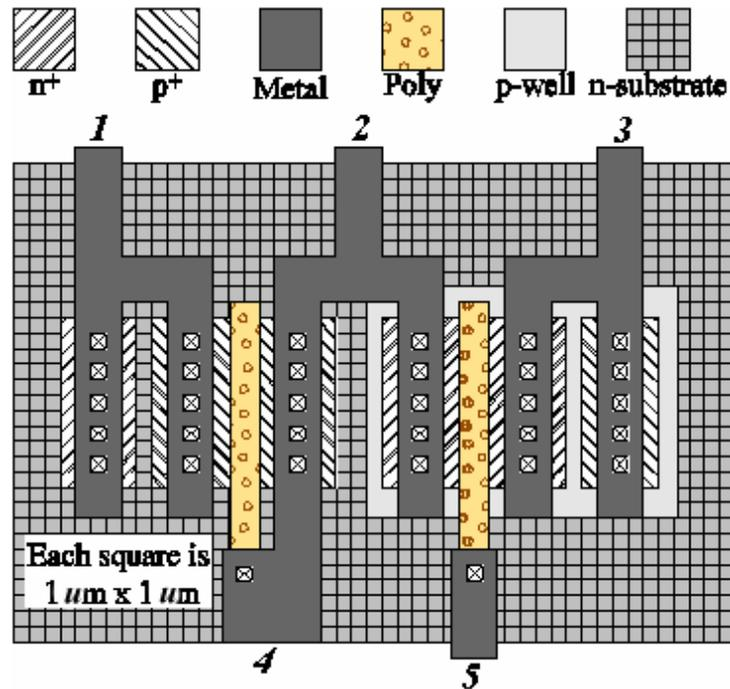
(b) Which terminal(s) (1, 2, 3, 4, or 5) is(are) more than likely connected to the positive power supply?
